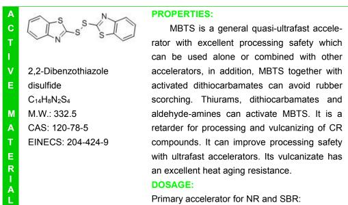
1.0-2.0phr with 2.0-3.0phr sulfur; for IIR: 0.25-1phr with 1-2phr sulfur.
